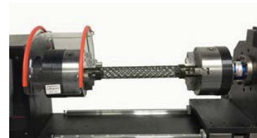
Fig.2. Tube torsion test.
